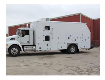
Single and tandem axle heavy duty Wireline units for cased hole service applications. Units are designed to operate in rough terrain environments. Trucks are fitted with air ride suspension to lesson shock load during transportation on rough roadways. Precise is a custom manufacturer that can build these units in any configuration required by our customers. Every Precise customer has final design approval prior to construction implementation of their equipment.
